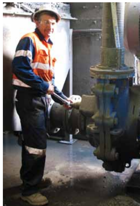
Paul Sharp from Sibelco Australia's Tallawang site in NSW, Australia, adjusts the revolutionary new Warman® WBH® pump without stopping production.
