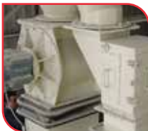
Airtight discharge valve to avoid air intake that could affect the classification performance.
